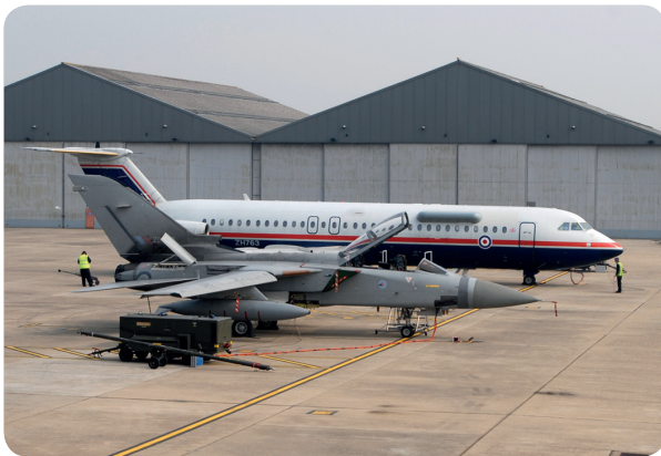
Figure 1: QinetiQ's Tornado and BAC 1-11 aircraft QinetiQ's Tornado and BAC 1-11 aircraft used during the surrogate UAV flight trials which used a dedicated Kontron multi form factor system based on 3U CompactPCI® and VME.
