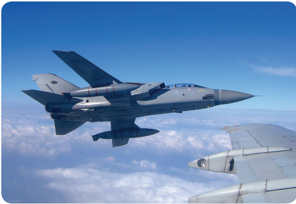
Figure 2: QinetiQ's Tornado Integrated Avionics Research Aircraft (TIARA) pictured from its BAC 1-11 which was acting as a surrogate UAV as part of the overall trial
