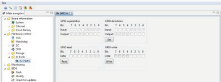
Figure 12: Configuring GPIO Pins using JIDA32/K-Station
