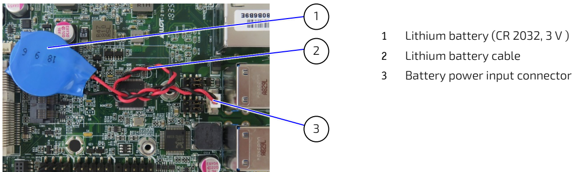
Figure 43: Lithium Battery Power Input Connector
