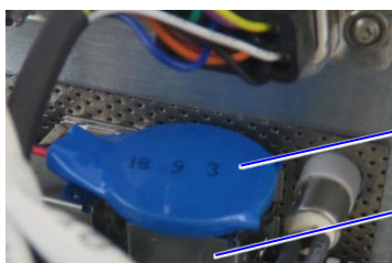
Figure 42: Lithium Battery Location
