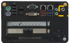
Figure 10: 12 VDC Power Jack
