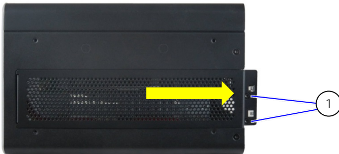
Figure 25: PCIe Expansion Card Screws
