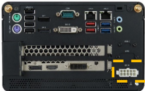
Figure 13: DC_IN 24 VDC 10-Pin Connector
