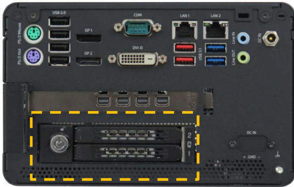
Figure 18: Storage Bay with Dual Removable 2.5" SSDs
